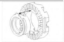
**22.** Verify paddle opening (widest gap) in other synchroring is facing the back of the differential, away from you.
