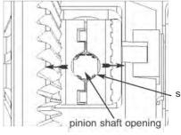
**37.** Feel through pinion shaft opening and verify both spacers and drivers are fully seated onto couplers. Verify all 8 saddle springs are fully seated in holes.
