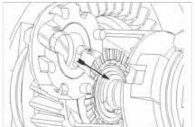
**19.** Insert driver/spacer as shown, making sure spacer paddle is facing out towards you.
