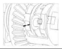
**35.** Insert 2nd c-clip through c-clip slot in driver onto axle shaft; pull axle shaft out to seat c-clip.
