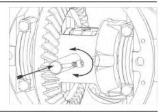
**40.** Insert retaining bolt/roll-pin into case/shaft. Tighten retaining bolt firmly.
