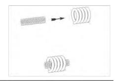
**27.** Compress inner spring and install spring assembly into spring slot.
