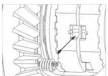
**30.** Compress inner spring and install the second spring assembly into the second spring slot.
