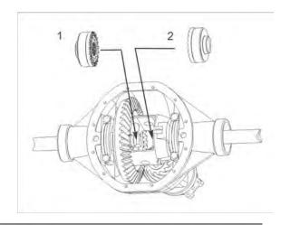
**16.** Install c-clip on ring gear side axle shaft only.
