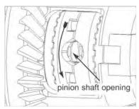
**36.** Making sure drivers stay engaged with couplers, carefully rotate both wheels backwards 1/4 turn to expose pinion shaft opening.
