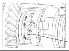
**29.** Keeping both drivers wedged in engagement with couplers, rotate driver's side wheel forward 1/2 turn to reveal spring slot on other side.
