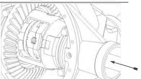
**34.** Making sure drivers stay engaged with couplers, carefully rotate driver's side wheel until c-clip slot is accessible. Verify c-clip groove on axle is accessible through c-clip slots on driver and spacer.
