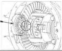
**23.** Install slotted driver/spacer making sure that paddle is pointing away from you toward rear of differential.
