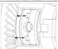
**24.** Verify spacer paddle is aligned with the paddle opening in synchro ring and press down on driver /spacer to seat on coupler; driver teeth should be fully engaged all the way around.
