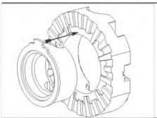
**18.** Insert the non-slotted spacer into the non-slotted driver. Seat the spacer paddle at the missing extended tooth.
