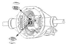
**11.** Remove side gears, clutches, and thrust washers.
