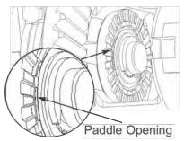
**17.** Make sure paddle opening (widest gap) in ring gear side synchro ring is facing out towards you.
