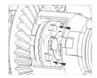
**21.** Insert the slotted spacer into the slotted driver. Seat the spacer paddle at the missing extended tooth.
