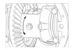
**39.** Using the retaining bolt/roll-pin as a handle, insert the shaft into the differential. Press hard while twisting to pass shaft by springs.
