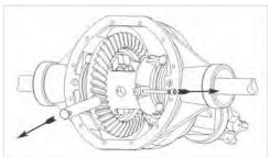
**7.** Expose pinion shaft;remove retaining bolt/roll pin and shaft.
