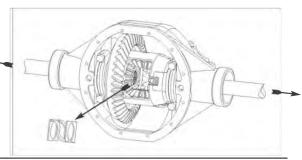
**10.** Remove both spider gears and their thrust washers.
