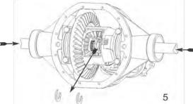
**8.** Push both axles inward and remove both c-clips. Remove o-rings from c-clip grooves on axle shafts if present.
