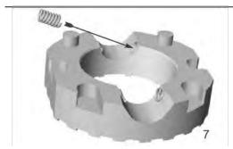
**14.** Apply wheel bearing grease to saddle springs & seat in holes.
