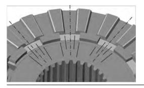
**12.** Verify gaps in coupler teeth are positioned within gaps in synchro ring. Place coupler in a vise and use an active spacer to align them if necessary.
