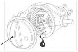
**6.** Remove differential cover and drain fluid. Clean the diff cover and housing sealing surface.
