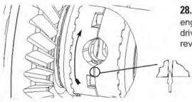
**28.** Keeping both drivers wedged in engagement with couplers, rotate drivers/couplers forward 1/2 turn to reveal spring slot on other side.
