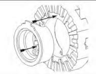
21. Verify paddle opening (widest gap) in other synchro ring is facing the back of the differential, away from you.
