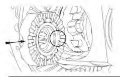
22. Install second driver/spacer making sure that paddle is pointing away from you toward rear of differential.
