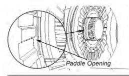
**16.** Make sure paddle opening (widest gap) in ring gear side synchro ring is facing out towards you.
