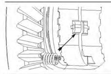
**29.** Compress inner spring and install the second spring assembly into the second spring slot.
