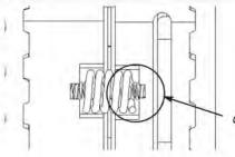
**30.** Visually inspect notches in spring slot to make sure inner spring is fully seated.
