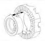
17. Insert an active spacer into a driver. Seat the spacer paddle at the paddle opening in the driver (missing extended tooth).
