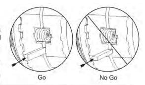
**32.** Keeping both drivers fully engaged with couplers, rotate drivers/couplers back 1/4 turn to expose pinion shaft opening.
