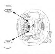
**10.** Remove both sidegears and thrust washers.
