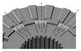
11. Verify gaps in coupler teeth are aligned with gaps in synchro ring. Place coupler in a vise and use an active spacer to align them if necessary.
