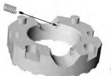
**13.** Apply wheel bearing grease to saddle springs and seat in holes.
