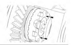
**20.** Insert the second active spacer into the second driver. Seat the spacer paddle at the paddle opening in the driver (missing extended tooth).
