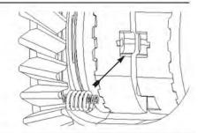
**27.** Visually inspect notches in spring slot to make sure inner spring is fully seated.
