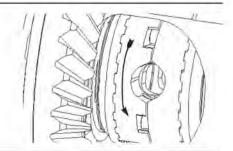
33. Feel through pinion shaft opening and verify both spacers and drivers are fully seated onto couplers. Verify all 8 saddle springs are fully seated in holes.
