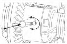
**35.** Using the retaining bolt/roll-pin as a handle, insert the shaft into the differential. Press hard while twisting to pass shaft by springs.
