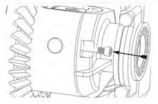
**36.** Insert retaining bolt/roll-pin into case/shaft. Tighten retaining bolt firmly.
