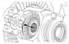
**18.** Insert driver/spacer as shown, making sure spacer paddle is facing out towards you.
