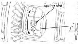
**24.** Wedge both drivers in engagement with couplers. Rotate drivers/couplers forward 1/4 turn to reveal spring slot.
