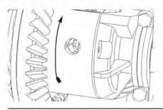
**34.** Keeping couplers and drivers stationary, rotate case 1/4 turn forward to align pinion shaft openings.
