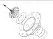
**16.** Remove the second sidegear and thrust washer.
