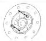
28. Place the two spring assemblies into the spring holes (holes with a step) in the driver.
