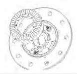
**30.** Install the second coupler into the differential case. Make sure paddle opening (widest gap) in synchro ring is aligned with the block's paddle. The driver and coupler teeth should be fully engaged.
