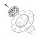
21. Insert the block onto the coupler making sure the block's paddle is aligned with the paddle opening (widest gap) in the synchro ring.
