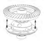
12. Remove the smaller half (cap) of the differential case. The case halves should have been marked in Step 11 as they must be reinstalled in their original position.
