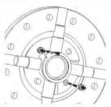
27. Place the two spring assemblies into the spring holes (holes with a step) in the driver.
