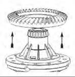
13. Remove the smaller half (cap) of the differential case. The case halves should have been marked in Step 12 as they must be reinstalled in their original position.
