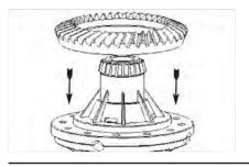
**31.** Install the ring gear back onto the case. Make sure the mark on the ring gear lines up with the mark on the two halves of the case.
