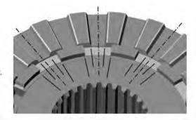
**18.** Apply wheel bearing grease to driver teeth.
