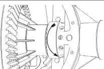
**10.** Loosen the bearing adjusters.
