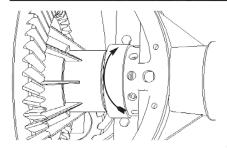
**33.** Tighten bearing adjusters back to their original positions.
