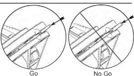
**25.** If the gap is correct, remove the cap, gage ring, and coupler to proceed.
