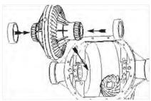
**32.** Place the bearing races on the corresponding bearings and install the assembly in the third member.
