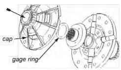
24. Check the gap in the differential case using the gage block. The narrow side of the block should fit in the gap, but the wider side should not fit.
