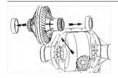
11. Pull out the differential case from the third member. Remove the bearing races from the bearings and mark them. The bearing races must be installed on the same bearings they were originally on to avoid bearing failure.
