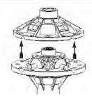
14. Remove the side gear and thrust washer.
