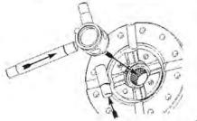
22. Insert the pinion shafts into the block (small diameters facing outwards) and insert the block with the pinion shafts into the case. Make sure the block's paddle passes through the driver notch and seats in the paddle opening (widest gap) in the synchro ring.
