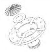
**16.** Remove the second side gear and thrust washer.
