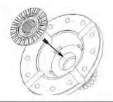
20. Install a coupler into the case.
