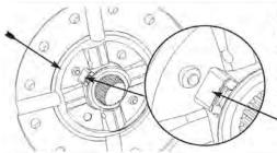
21. Insert the driver onto the coupler making sure the driver's notch is aligned with the paddle opening (widest gap) in the synchro ring.
