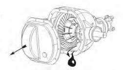
Remove axle shafts from housing.
