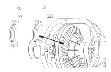
35. Reinstall axle shafts in housing.
