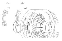
9. Remove adjuster locks and bearing caps from the housing. These parts should have been marked in Step 8 as they are not interchangeable and must be reinstalled in their original positions.
