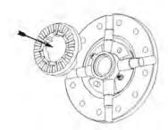
29. Install the second coupler into the differential case. Make sure paddle opening (widest gap) in synchroring is aligned with the block's paddle.
