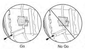
**31.** Check the gap between drivers using check block. The narrow side of the block should fit between the drivers, but the wider side should not fit.
