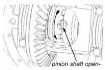
36. Feel through pinion shaft opening and verify both spacers and drivers are fully seated onto couplers. Press down on thrust slugs so that they are seated against the axle ends. Verify all 8 saddle springs are fully seated in saddle springs holes.
