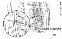
**21.** Verify paddle opening (widest gap) in other synchro ring is facing the back of the differential, away from you.
