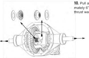
**10.** Pull axle shafts out approximately 6". Remove side gears and thrust washers.
