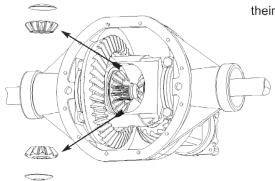
**9.** Remove both spider gears and their thrust washers.
