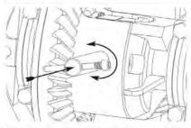
**38.** Using the retaining bolt as a handle, insert the shaft into the differential. Press hard while twisting to pass shaft by springs.
