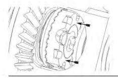
**19.** Verify spacer paddle is aligned with paddle opening in synchro ring and press driver/spacer down onto coupler. Driver teeth should be fully engaged all the way around.
