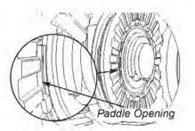
17. Insert the thrust slug into the non-slotted spacer. Insert the nonslotted spacer/thrust slug into the non-slotted driver. Seat the spacer paddle at the paddle opening in driver (missing extended tooth).
