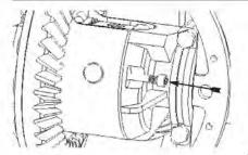
**39.** Insert retaining bolt into case/shaft. Tighten retaining bolt firmly.
