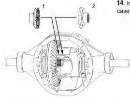
**14.** Install couplers inside differential case, ring gear side first.
