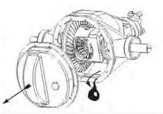
7. Expose pinion shaft; remove retaining bolt and shaft. Remove thrust block.
