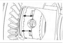
**24.** Wedge both drivers in engagement with couplers. Rotate driver's side wheel forward 1/4 turn to reveal spring slot.
