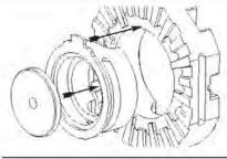
**20.** Insert the thrust slug into the slotted spacer. Insert the slotted spacer/thrust slug into the slotted driver. Seat the spacer paddle at the paddle opening in driver (missing extended tooth).
