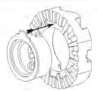
21. Insert the second active spacer into the second driver. Seat the spacer paddle at the paddle opening in driver (missing extended tooth).
