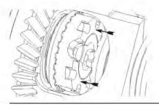
**20.** Verify spacer paddle is aligned with paddle opening in synchro ring and press driver/spacer down onto coupler. Driver teeth should be fully engaged all the way around.
