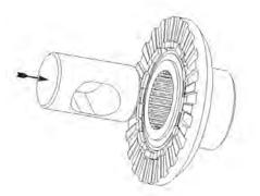
**15.** Insert the thrust block into the coupler that will go on the axle shaft opposite the ring gear.
