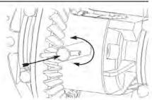
37. Drive roll-pin into case/shaft.
