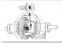
**10.** Remove passenger-side side gear/thrust block/thrust washer together. Retain thrust block.
