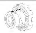
19. Insert driver/spacer as shown, making sure the spacer paddle is facing out towards you.
