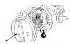
7. Expose pinion shaft; use a punch to drive out roll pin. Remove pinion shaft.
