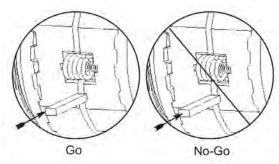
32. Check the gap between drivers using check block. The narrow side of the block should fit between drivers, but the wider side should not fit. If gap is incorrect, STOP and call
