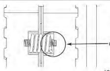
**28.** Visually inspect notches in spring slot to make sure inner spring is fully seated.
