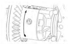
**36.** Using the roll-pin as a handle, insert the shaft into the differential. Press hard while twisting to pass shaft by springs.
