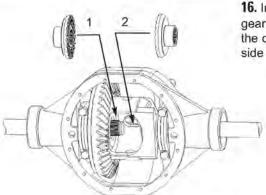
**16.** Insert the coupler into the ring gear side of the case first. Insert the coupler with thrust block into the side opposite the ring gear.
