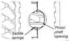
34. Keeping both drivers fully engaged, rotate both wheels back 1/4 turn to expose pinion shaft opening. Make sure saddle springs are all fully seated and the pinion shaft opening in the thrust block is aligned with the pinion shaft opening in the drivers.
