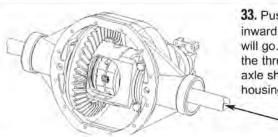
33. Push passenger side axle shaft inward through coupler as far as it will go. The axle shaft should push the thrust block against the opposite axle shaft. Bolt axle shaft back to housing.
