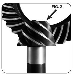
**NOTE:** If measured clearance of less than 0.5mm (0.020") between the GRIP unit and the pinion gear exists, then unwanted contact between the two could occur when the assembly flexes under high torque application.
