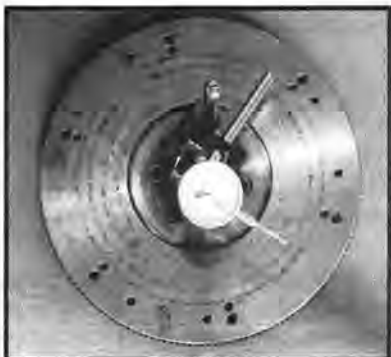
This is how the dial indicator must be positioned to check concentric alignment of the rear bellhousing opening with the crankshaft centerline.
