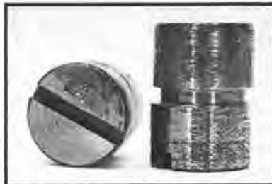
Shown is a pair of the offset dowel pins, along with two 10-32 set screws to lock the dowels in place when the alignment process is completed.
